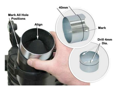
Apply adhesive sealant to the steel adaptor (item 11) and to the inside of the air cleaner inlet housing.
