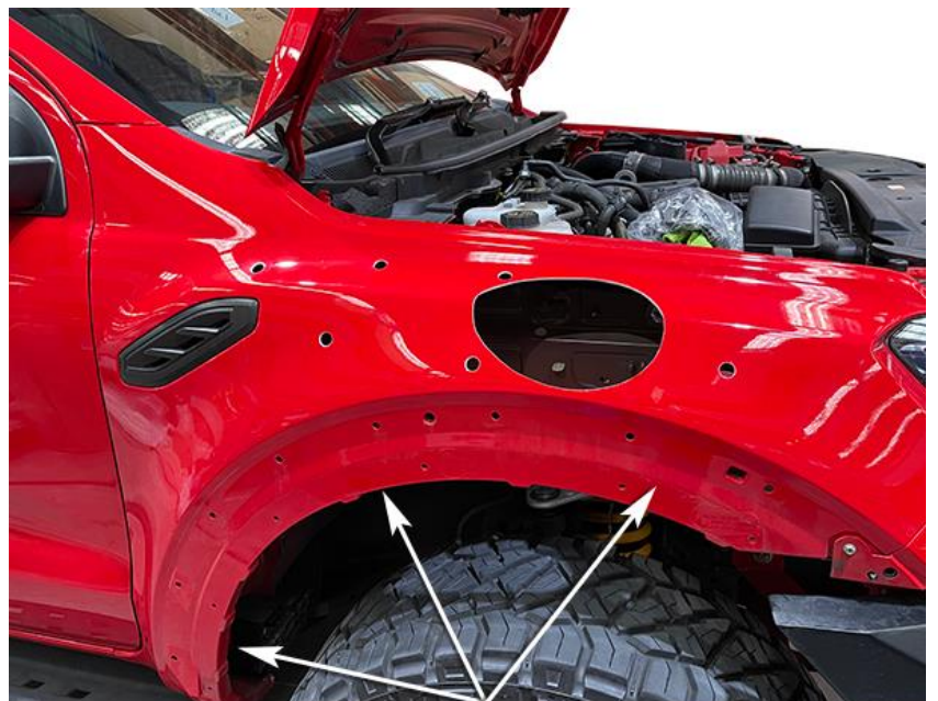
Fender Flare & Inner Guard Liner Removed
