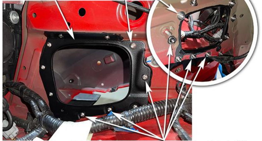
M5 x 12mm B/H Bolts w/ Body Washers & Nyloc Nuts (x10)
