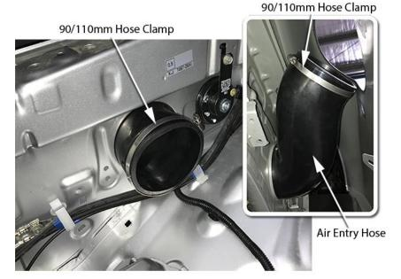
Re-install the air cleaner base, guiding the air cleaner inlet into the air entry hose, fasten the air cleaner base using standard mounting bolts.
