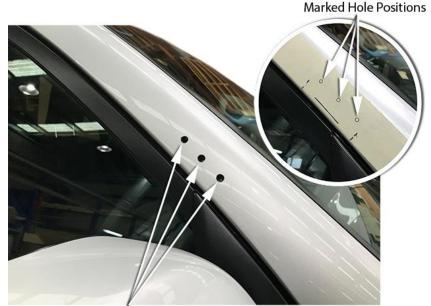
Drilled Holes 8mm Dia
