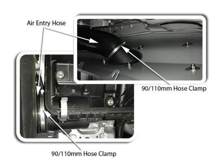
Loosely install the black hose clamp (Item 12) over the base of the air ram assembly (Item 2).
