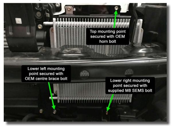
19. Remount the OEM horn to the top left leg of the cooler bracket.
