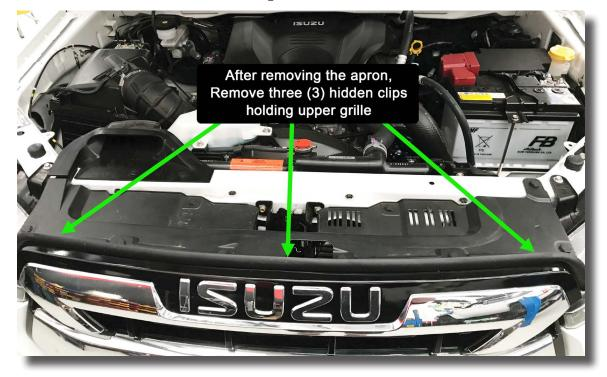
5. Remove the (1) phillips head screw in the centre of the grill located just under the Isuzu front badge.
