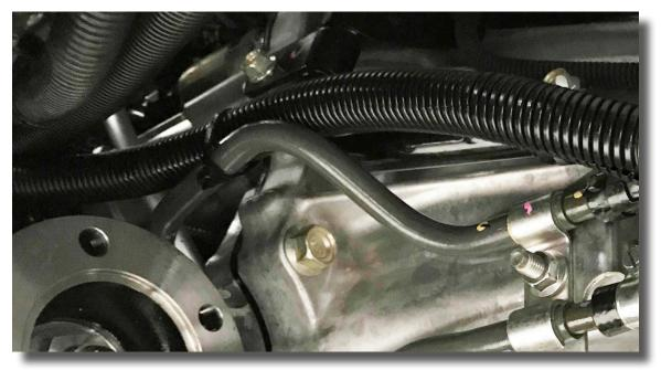
Run the cooler line down beside transmission and existing cooler lines and 24. connect to centre outlet on OEM heat exchanger. Secure with supplied screw clamp.
