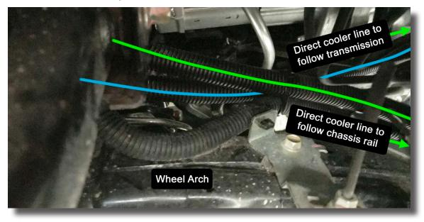
Remove OEM hose that joins the steel line on side of transmission with 22. centre outlet in heat exchanger. This can be discarded.
