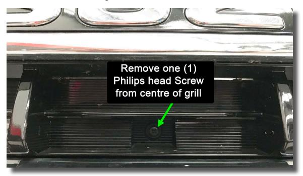
6. Remove top half of the grill by firmly pulling forwards. Set aside.
