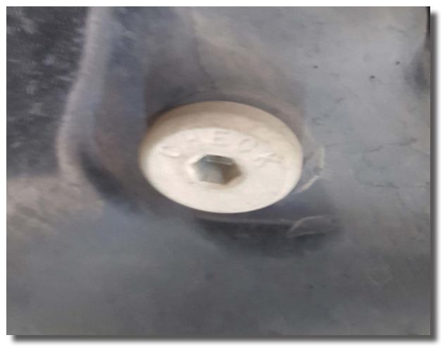
33. With the **engine running**, remove using a 5mm Allen key. DO NOT remove the 14mm bolt located at the rear of the transmission pan as this is the drain plug.
