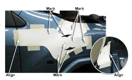
Trim Step Drill 16mm Dia Drill 98mm Dia Deburr & Paint
