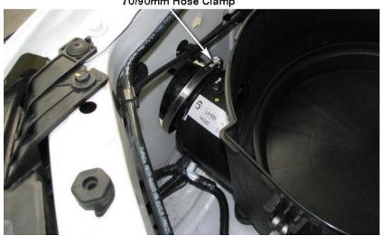
Loosely install a 70/90mm hose clamp (Item 11) over the air cleaner inlet adaptor, install the air cleaner base into the vehicle and fasten with standard mounting bolts.
