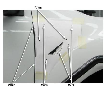
Step Drill 16mm Dia Marked Hole Positions
