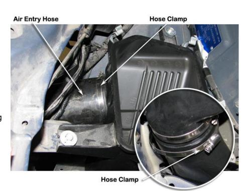
Support the connection hose and air entry hose assembly in position with a 360mm long cable tie (Item 16) as shown.
