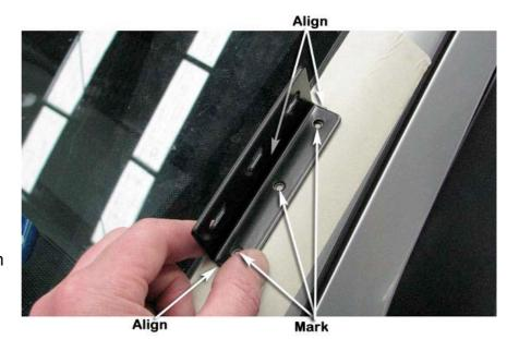
Drill a pilot hole at each of the three marked hole positions. Drill each hole position to 8mm diameter with a step drill or 8mm drill bit.
