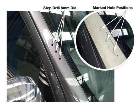
Drill a pilot hole at each of the three marked hole positions. Drill each hole position to 8mm diameter with a step drill or 8mm drill bit.
