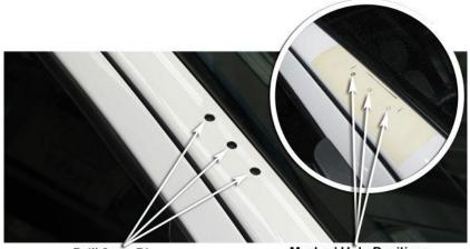
Drill 8mm Dia Marked Hole Positions
